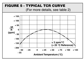
**Note:** The TCR values for  $< 80~\Omega$  are influenced by the termination composition and the result in deviation from this curve
