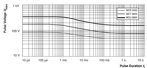
Maximum pulse voltage, single and continuous pulses; for permissible resistance change equivalent to 8000 h operation **Pulse Voltage**
