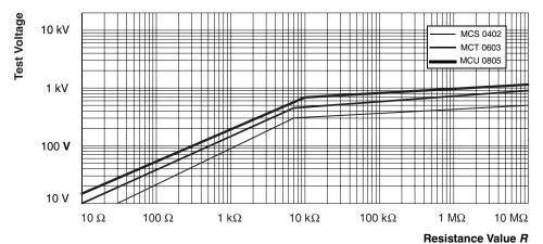
Pulse load rating in accordance with EN 60115-1 clause 4.27; 10  $\mu$ s/700  $\mu$ s; 10 pulses at 1 min intervals; for permissible resistance change 0.5 %
