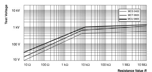
Pulse load rating in accordance with EN 60115-1 clause 4.27; 1.2 μs/50 μs; 5 pulses at 12 s interval; for permissible resistance change 0.5 %
