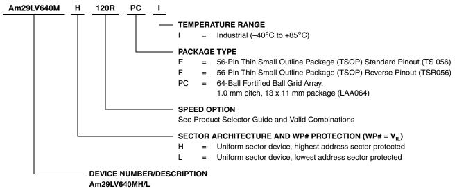
64 Megabit (4 M x 16-Bit/8 M x 8-Bit) MirrorBit™ Uniform Sector Flash Memory with VersatileIO™ Control, 3.0 Volt-only Read, Program, and Erase
