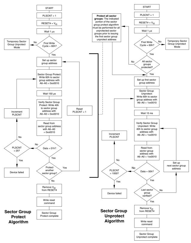
Figure 2. In-System Sector Group Protect/Unprotect Algorithms
