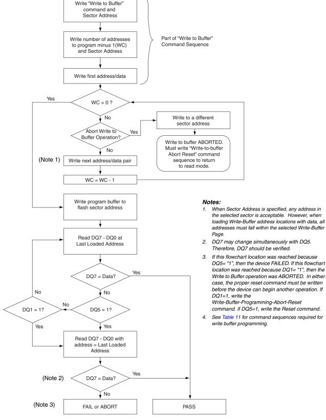
Figure 4. Write Buffer Programming Operation
