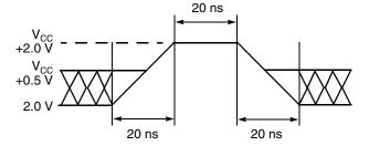
Figure 10. Maximum Negative **Overshoot Waveform**
