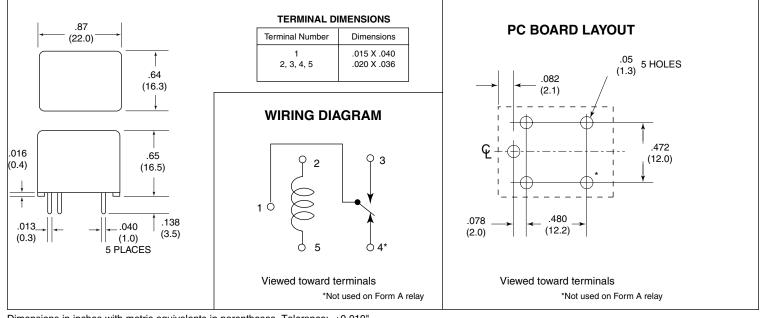
Dimensions in inches with metric equivalents in parentheses. Tolerance: ±0.010"
