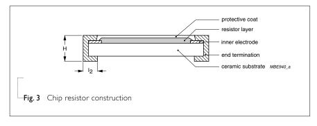
resistance value. Finally, the two external terminations (pure Tin) are added. See fig. 3.
