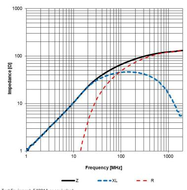
Test Equipment: E4991A or equivalent
