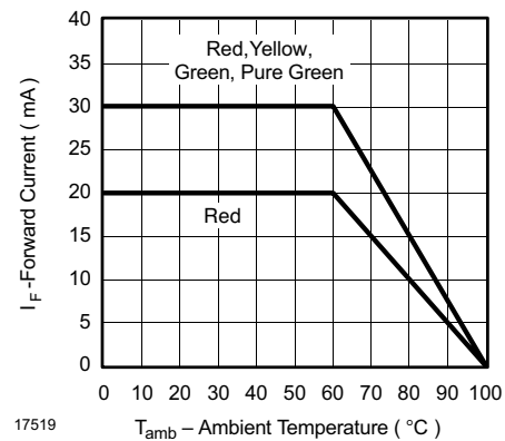
Figure 2. Forward Current vs. Ambient Temperature
