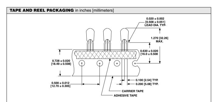
**Tape and Reel Specifications:** Type 299D radial-leaded tantalum capacitors are available taped and reeled per EIA-468.
