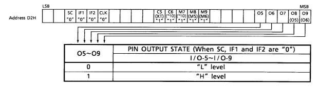
Note 22: On TC9257P and TC9257F, pins I/O-7~I/O-9 also serve as general-purpose counter input pins. Therefore, bits SC, IF1 and IF2 of the input register (D2H) must be set to "0" when pins I/O-7~I/O-9 are used for I/O ports. Since pin I/O-5 also serves as the CLK pin, the CLK bit of the input register (D2H) must be set to "0" when pin I/O-5 is used as an I/O port.
