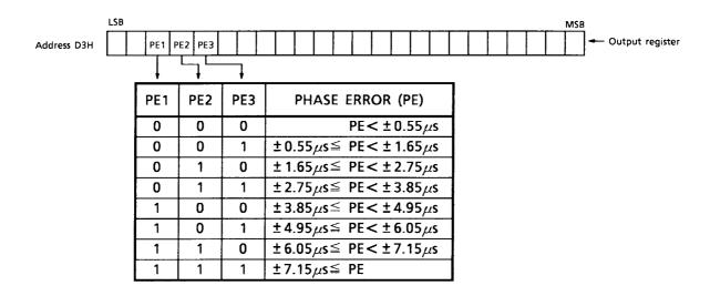
The phase error data can be read from the output register (D3H) as serial data PE1~PE3.
