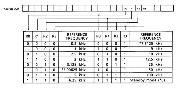
Note 8: Reference frequencies marked with an asterisk "\*" can only be generated with a 4.5 MHz crystal oscillator.
