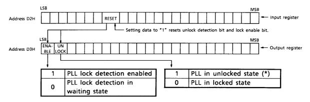
Note 31: The asterisk "(\*)" indicates an error state of over 180° phase difference relative to the reference frequency.
