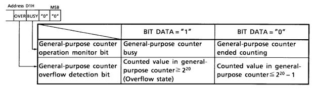
Note 17: When using the general-purpose counter, before referring to the contents of the general-purpose counter result bits (f0~f19), confirm that the BUSY bit is "0" (counting is ended) and the OVER bit is "0" (general-purpose counter data are normal).
