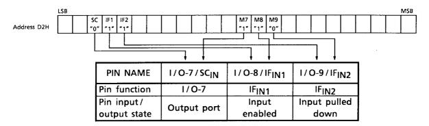
As shown above, the pins can be switched as necessary to enable use as an  $I\!/O$  port or general-purpose counter.
