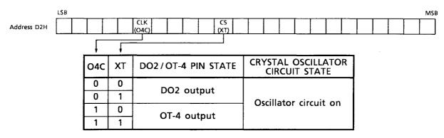
2. DOHZ Bit......Controls the DO2 Pin output state.
