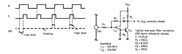
Figure 8 DO Output Timing Chart
