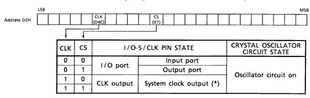
Note 32: The system clock output marked with an asterisk "(\*)" refers to output of the crystal oscillator frequencies listed below.
