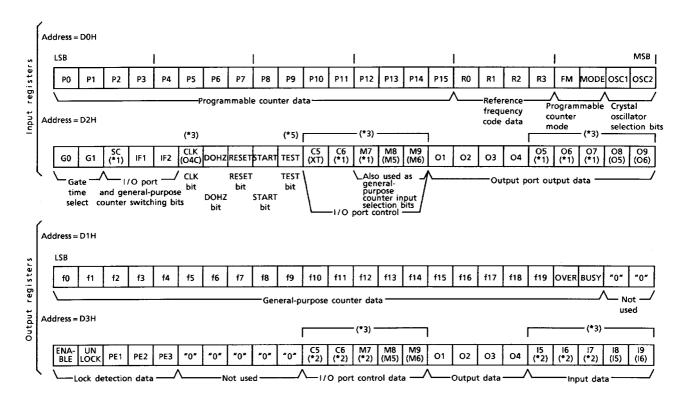
When power is turned on, the input registers are set as shown below.
