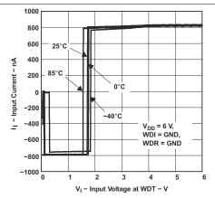
Figure 7-4. Input Current vs Input Voltage at WDT
