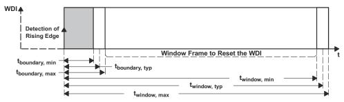
Figure 8-2. Upper and Lower Boundary Visualization
