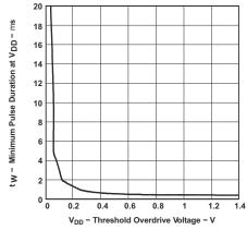
Figure 7-6. Minimum Pulse Duration at V<sub>DD</sub> vs V<sub>DD</sub> Threshold Overdrive Voltage
