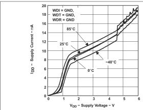
Figure 7-2. Supply Current vs Supply Voltage
