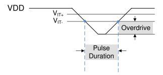
Figure 8-1. Overdrive Versus Pulse Duration
