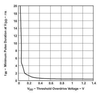
Figure 9-2. Minimum Pulse Duration at V<sub>DD</sub> vs V<sub>DD</sub> Threshold Overdrive Voltage
