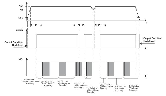
Figure 7-1. Timing Diagram
