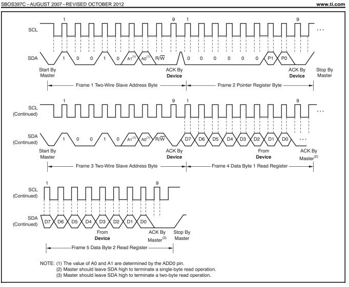
Figure 14. Two-Wire Timing Diagram for Read Word Format
