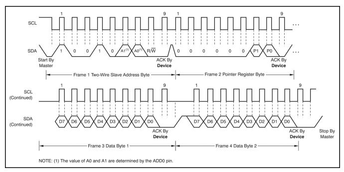
Figure 13. Two-Wire Timing Diagram for Write Word Format
