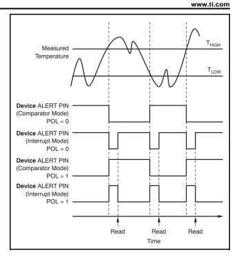
Figure 10. Output Transfer Function Diagrams
