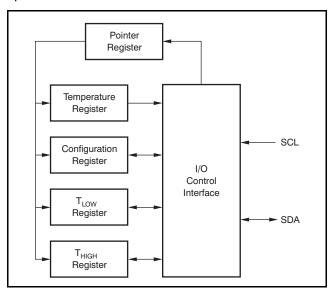
Figure 8. Internal Register Structure
