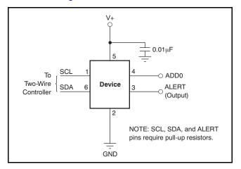
Figure 7. Typical Connections
