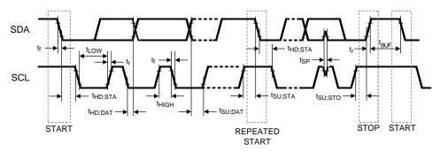
Figure 1. I<sup>2</sup>C Timing
