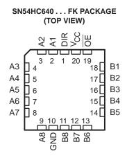
SN54HC640, SN74HC640 OCTAL BUS TRANSCEIVERS WITH 3-STATE OUTPUTS SCLS303D – JANUARY 1996 – REVISED AUGUST 2003
