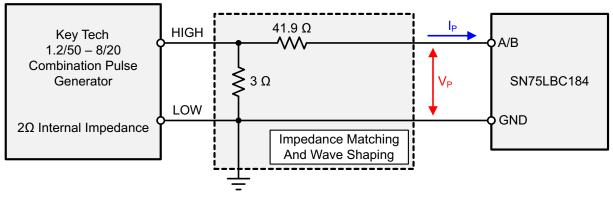
Figure 19. Overvoltage Stress Test Circuit
