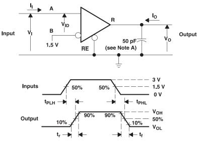
A. This value includes probe and jig capacitance (±10%).
