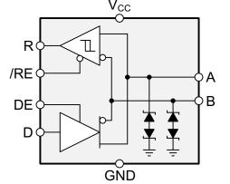
Figure 13. Functional Logic Diagram
