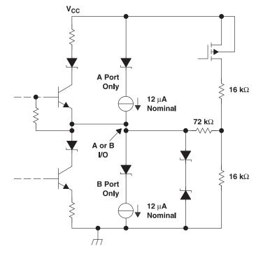
Figure 14. Schematic of Inputs and Outputs
