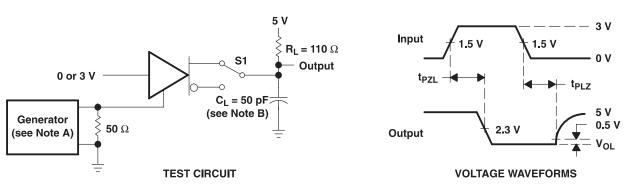
Figure 6. Driver t<sub>PZH</sub> and t<sub>PHZ</sub> Test Circuit and Voltage Waveforms
