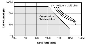
Figure 17. Cable Length vs Data Rate Characteristic
