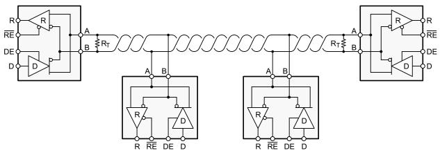
Figure 16. Typical RS-485 Network With Half-Duplex Transceivers
