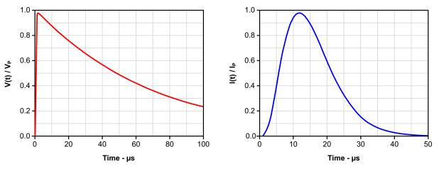
Figure 18. Open-Circuit Voltage and Short-Circuit Current Waveforms
