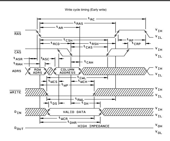
FIGURE 4. Switching waveforms - Continued.
