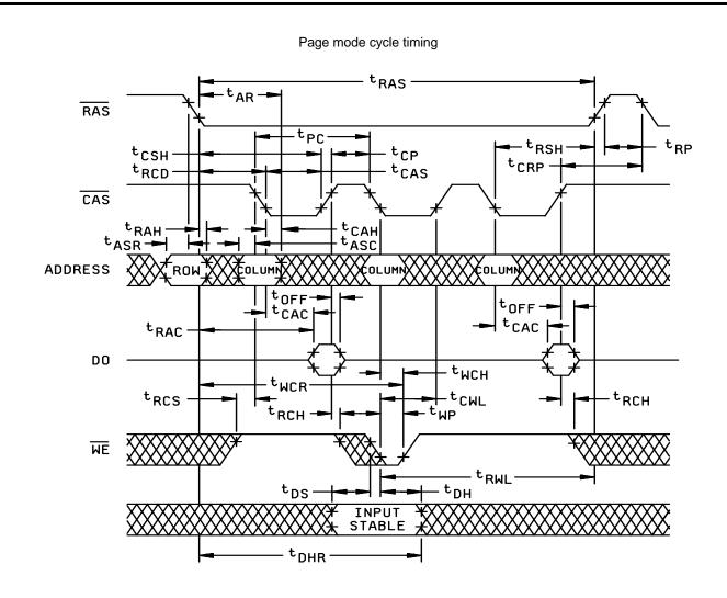
FIGURE 4. Switching waveforms - Continued.
