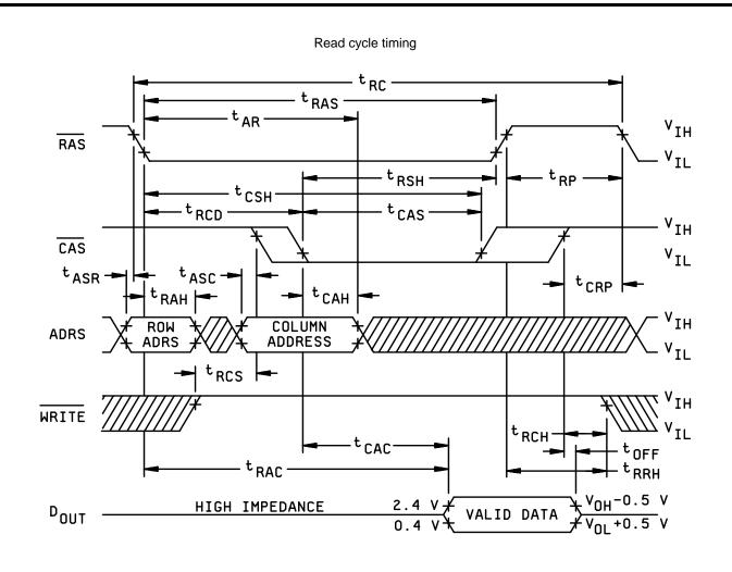
FIGURE 4. Switching waveforms.
