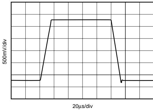
LARGE-SIGNAL STEP RESPONSE G = +1\text{V/V} , R_L = 100\text{k}\Omega , C_L = 100\text{pF}
