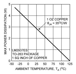
Figure 27. Maximum Power Dissipation vs. T<sub>AMB</sub> for the DDPAK/TO-263 Package
