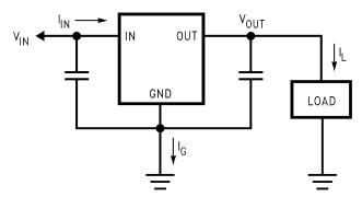
$$\begin{split} I_{IN} &= I_L + I_G \\ P_D &= (V_{IN} - V_{OUT}) \ I_L + (V_{IN}) \ I_G \end{split}$$
