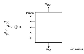
Measure inputs sequentially to both VDD and VSS. Connect all unused inputs to either VDD or VSS. Measure control inputs only.
