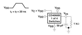
NOTES: A. All unused terminals are connected to  $V_{SS}$ .
