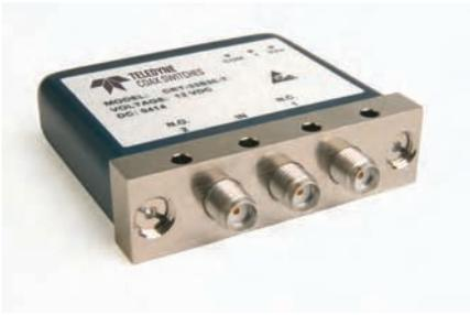
The CRT-33 Switch is an internally terminated, broadband, SPDT, electromechanical coaxial switch designed to switch a microwave signal from a common input to either of two outputs. The characteristic impedance is 50 Ohms. Internal terminations provide an impedance match for the unselected port. The switches are small with the minimum spacing that is compatible with SMA connectors.
