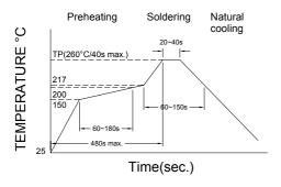
Figure 1. Re-flow Soldering
