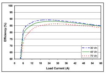
Figure 1: Efficiency at nominal output voltage vs. load current for minimum, nominal, and maximum input voltage at 25°C.
