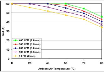
Figure 7: Maximum output power derating curves vs. ambient air temperature for airflow rates of 0 LFM through 400 LFM with air flowing from input to output (nominal input voltage).
