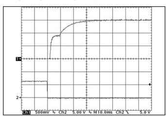
Figure 9: Turn-on transient at full load (resistive load) (10 ms/div). Input voltage pre-applied. Top Trace: Vout (0.5V/div). Bottom Trace: ON/OFF input (5V/div).
