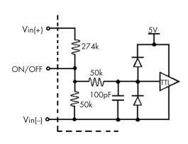
Figure B: Internal ON/OFF pin circuitry
