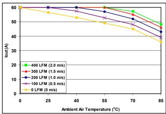
Figure 5: Maximum output power derating curves vs. ambient air temperature for airflow rates of 0 LFM through 400 LFM with air flowing from output to input (nominal input voltage).
