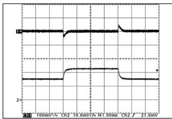
Figure 11: Output voltage response to step-change in load current (50%-75%-50% of Iout(max);  $dI/dt = 0.1A/\mu s$ ). Load cap:  $15\mu F$ , 450 m $\Omega$  ESR tantalum cap and 1µF ceramic cap. Top trace: Vout (100mV/div), Bottom trace: Iout (20A/div).
