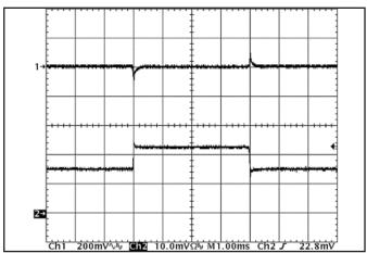
Figure 12: Output voltage response to step-change in load current (50%-75%-50% of Iout(max):  $dI/dt = 5A/\mu s$ ). Load cap:  $480\mu F$ , 15 m $\Omega$  ESR tantalum cap and 1µF ceramic cap. Top trace: Vout (200mV/div), Bottom trace: Iout (20A/div).
