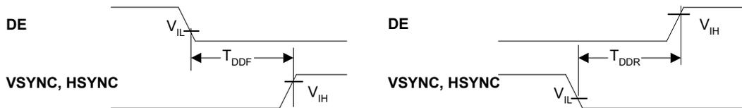
**Figure 5. VSYNC, HSYNC Delay Times to DE**
