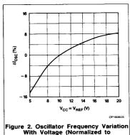
Figure 2. Oscillator Frequency Variation With Voltage (Normalized to  $V_{REF} = V_{CC} = 10V$ )  $T_A = +25^{\circ}C$
