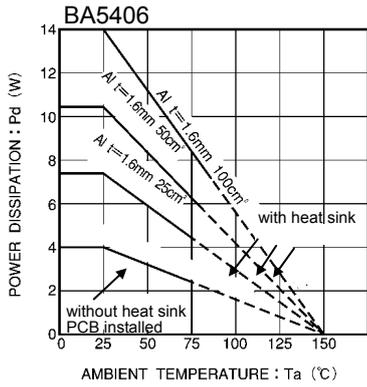
Fig.8 Thermal derating curve
