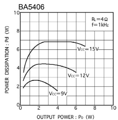
Fig.16 Power dissipation vs Output power(2)
