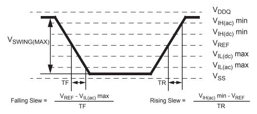
AC input test signal waveform
