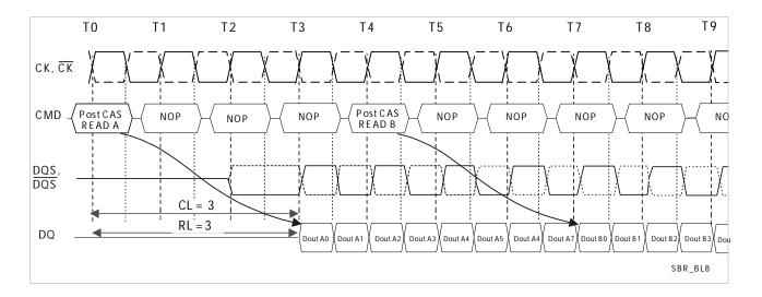
The seamless, non interrupting 8-bit burst read operation is supported by enabling a read command at every BL / 2 number of clocks. This operation is allowed regardless of same or different banks as long as the banks are activated.
