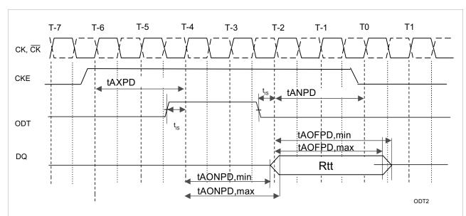
1) Both ODT to Power Down Entry and Exit Latencies tANPD and tAXPD are not met, therefore Power-Down Mode timings have to be applied.
