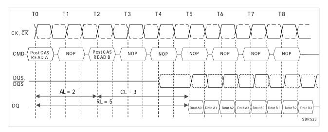
The seamless burst read operation is supported by enabling a read command at every BL / 2 number of clocks. This operation is allowed regardless of same or different banks as long as the banks are activated.
