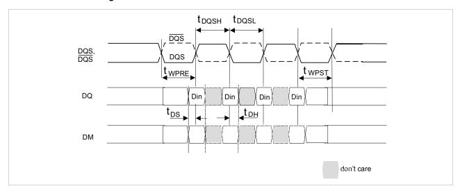
Burst Write Operation with Data Mask: RL = 3 (AL = 0, CL = 3), WL = 2, tWR = 3, BL = 4
