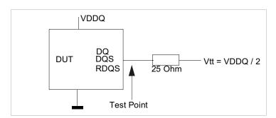
Output slew rate for falling and rising edges is measured between VTT - 250 mV and VTT + 250 mV for single ended signals. For differential signals (e.g. DQS -  $\overline{DQS}$ ) output slew rate is measured between DQS -  $\overline{DQS}$  = -500 mV and DQS -  $\overline{DQS}$  = +500 mV. Output slew rate is guaranteed by design, but is not necessarilty tested on each device.
