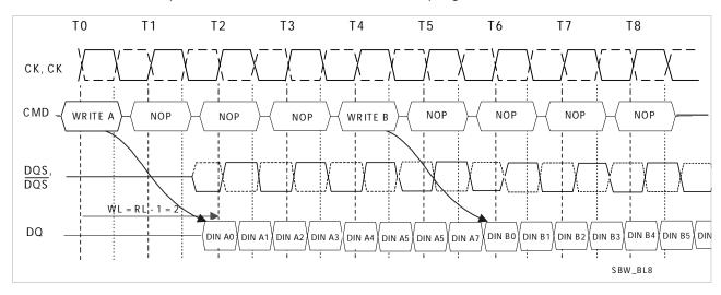
The seamless, non interrupting 8-bit burst write operation is supported by enabling a write command at every BL / 2 number of clocks. This operation is allowed regardless of same or different banks as long as the banks are activated.
