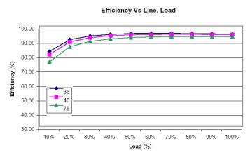
Figure 1. QKS48T21120 Efficiency vs. Output Load
