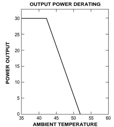
Typical Performance: ( $T_c=25^\circ\text{C}$ ,  $V_{in}=\text{Nom VDC}$ , Rated Load)
