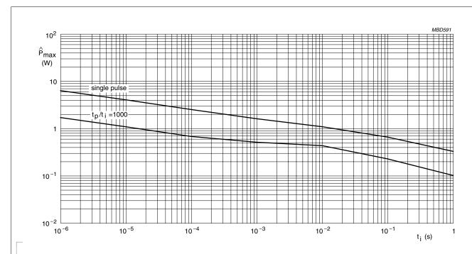
Fig. 8 Pulse on a regular basis for type: RC0603; maximum permissible peak pulse power as a function of pulse duration for single pulse and repetitive pulse tp/ti = 1000
