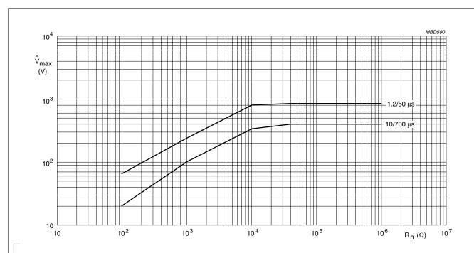
Maximum permissible peak pulse voltage without failing to open circuit' in accordance with DIN IEC 60040 (CO) 533 for type: RC0603
