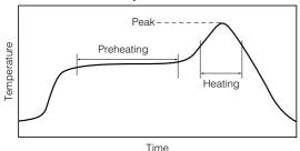
For soldering (Example: Sn/Pb)
