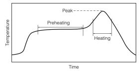
Recommended soldering conditions for flow
