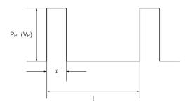
Withstand pulse limit power is calculated by the next method.
