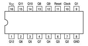
Figure 2. Pinout: 16-Lead Plastic Package (Top View)
