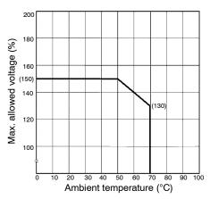
Note: The "Max. allowed voltage" is the maximum voltage that can be applied to the relay coil. It is not the maximum voltage that can be applied continuously.
