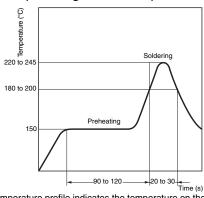
(The temperature profile indicates the temperature on the circuit board.)
