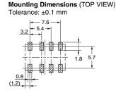
Note 1. Each value has a tolerance of ±0.3 mm. Note 2. The coplanarity of the terminals is 0.1 mm max.
