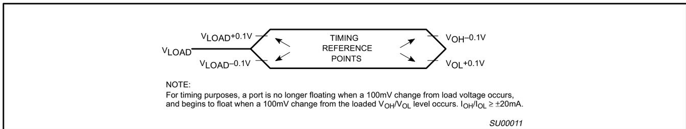
**Figure 24. Float Waveform**
