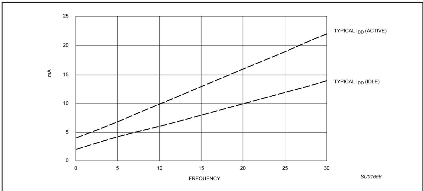
**Figure 28. I<sub>DD</sub> vs. Frequency at V<sub>DD</sub> = 3.0 V (typical)**
