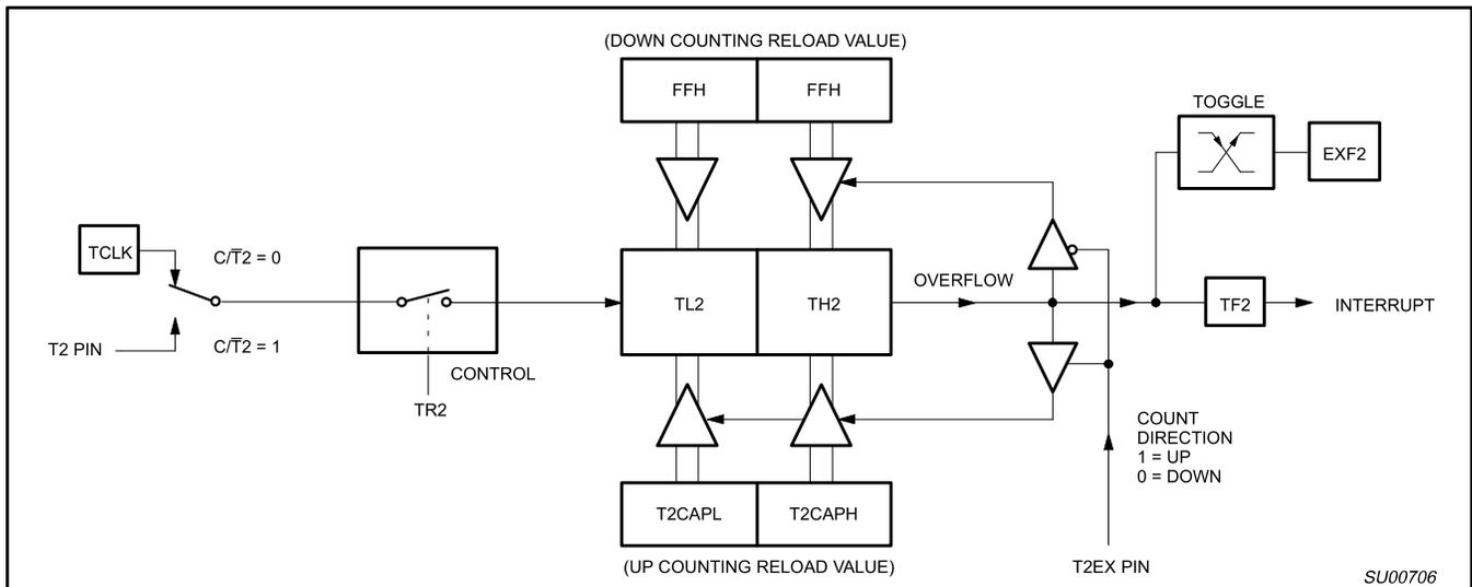
Figure 9. Timer 2 Auto Reload Mode (DCEN = 1)
