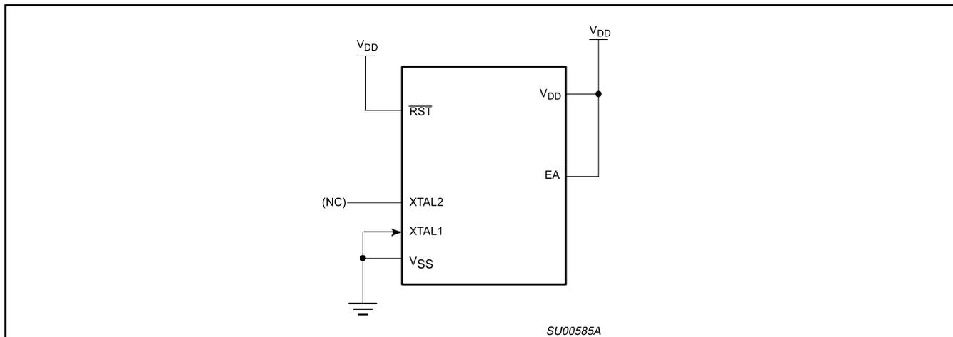
**Figure 30. I<sub>DD</sub> Test Condition, Power Down Mode**
