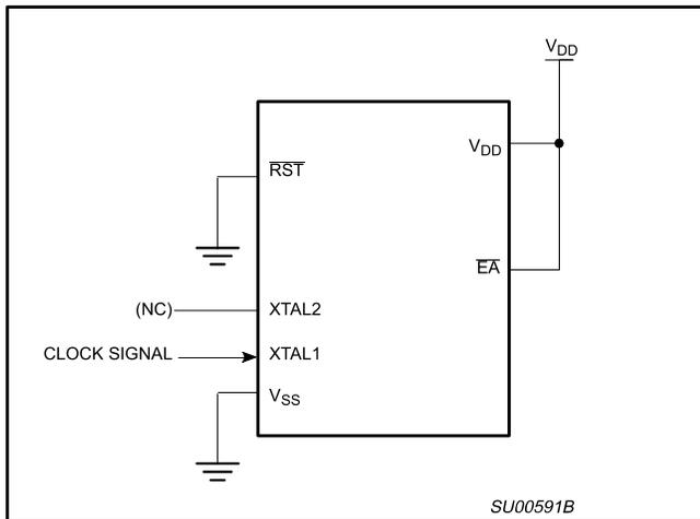
**Figure 25. I<sub>DD</sub> Test Condition, Active Mode**
