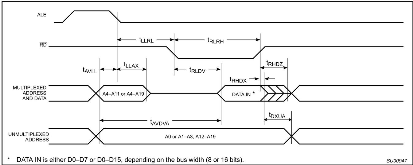
Figure 18. External Data Memory Read Cycle (ALE Cycle)
