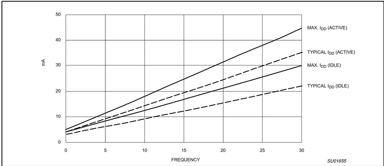
**Figure 27. I<sub>DD</sub> vs. Frequency at V<sub>DD</sub> = 5.5 V**
