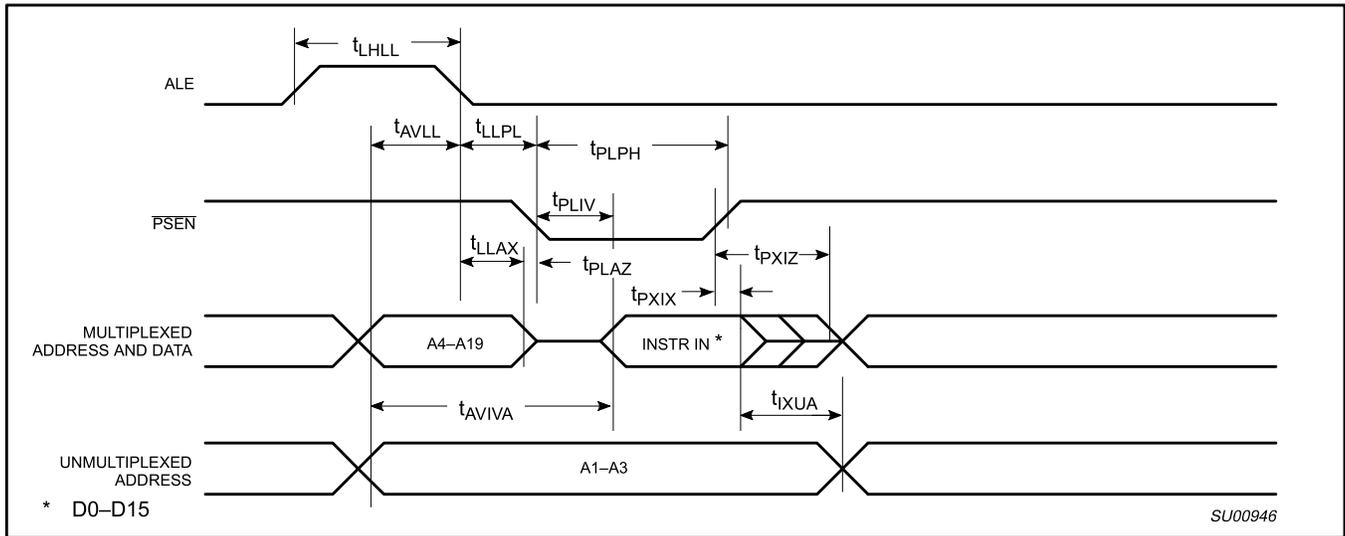
**Figure 16. External Program Memory Read Cycle (ALE Cycle)**
