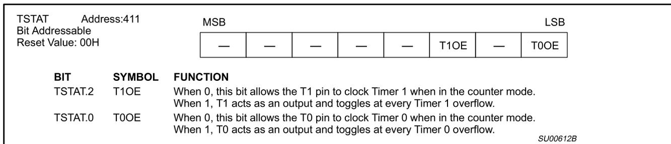
**Figure 5. Timer 0 And 1 Extended Status (TSTAT)**
