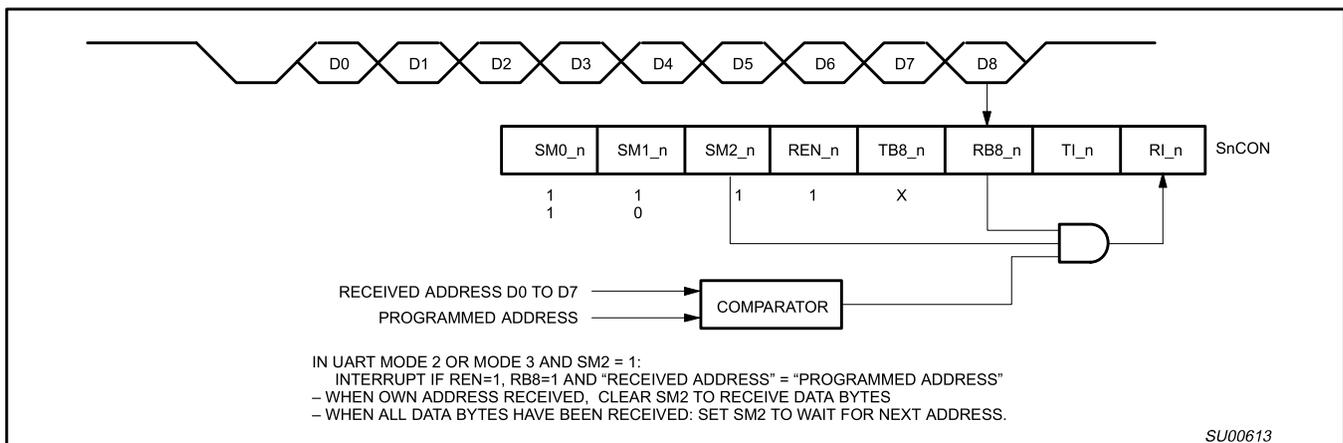
Figure 14. UART Multiprocessor Communication, Automatic Address Recognition
