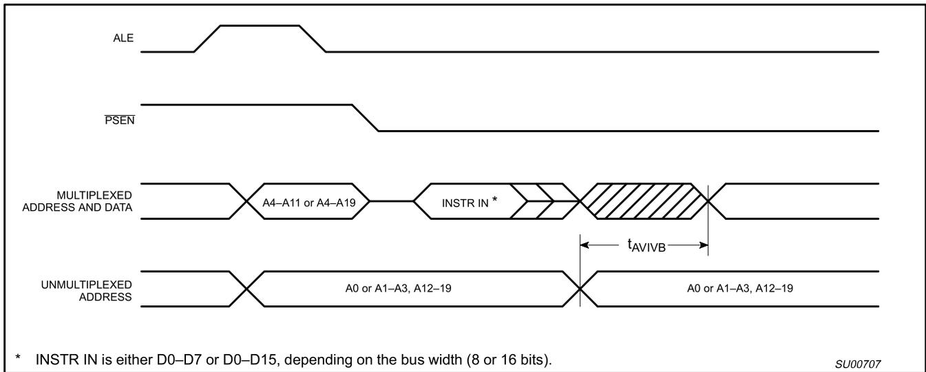
**Figure 17. External Program Memory Read Cycle (Non-ALE Cycle)**
