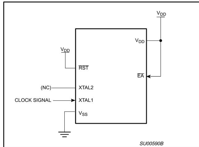
**Figure 26. I<sub>DD</sub> Test Condition, Idle Mode**
