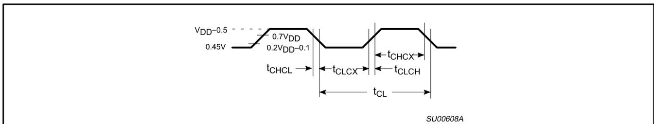
**Figure 29. Clock Signal Waveform for I<sub>DD</sub> Tests in Active and Idle Modes**
