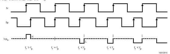
Note 15: fr is phase detector input from reference counter. fp is phase detector input from programmable N counter.
