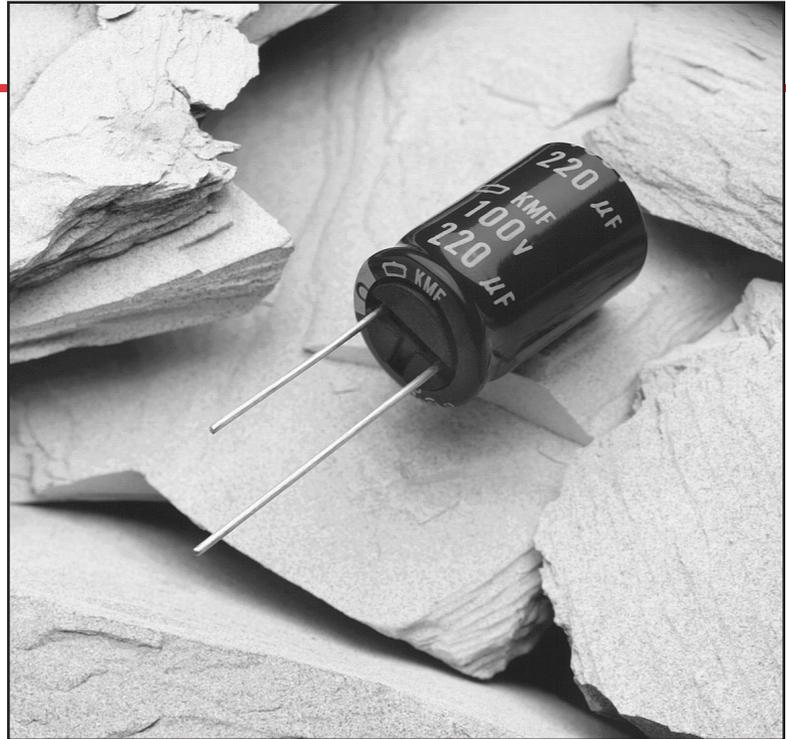
The KMF series capacitors are designed for low impedances at high frequencies with the case sizes of the KME general purpose capacitors. These capacitors will operate over a wide temperature range,  $-55^{\circ}\text{C}$  to  $+105^{\circ}\text{C}$ , with a load life of between 2,000 and 5,000 hours with the rated ripple current applied, depending on the case size.
