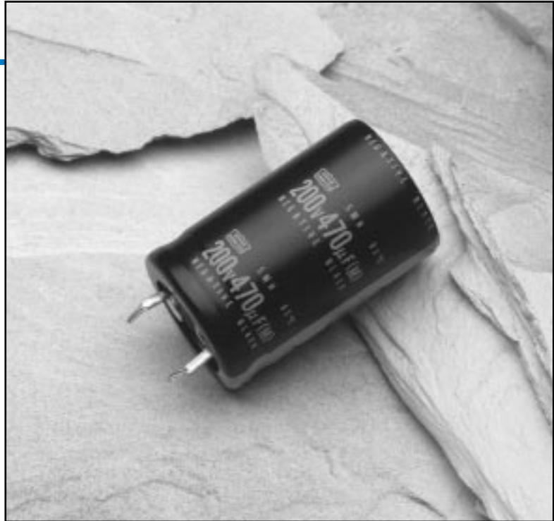
The SMH series capacitors are the standard 85°C, large capacitance, snap-in capacitors from United Chemi-Con. The load life for the SMH series is 2,000 hours at 85°C with the rated ripple current applied. The very high CV values and ripple current capabilities make these capacitors ideal for use in power supply filter circuits. The standard mounting style for the SMH series is a snap-in, 2-terminal configuration. Alternate 3, 4, and 5 pin terminal styles are available upon request.
