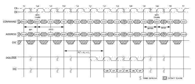
NOTE 1 Multipurpose registers Read/Write Enable (MR3 A2 = 1). Redirect all subsequent reads and writes to MPR locations.
