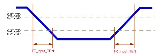
Single-Ended AC and DC Input levels for  $\overline{\text{CS}}$ , BA [1:0], BG [1:0], A [9:0], A10/AP, A12/ $\overline{\text{BC}}$ , A13,  $\overline{\text{WE}}$ /A14,  $\overline{\text{CAS}}$ /A15,  $\overline{\text{RAS}}$ /A16, CKE,  $\overline{\text{ACT}}$ , ODT, CK,  $\overline{\text{CK}}$ , and PAR
