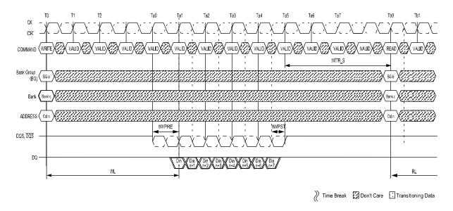
NOTE 1 tWTR\_S: Delay from start of internal write transaction to internal READ command to a different bank group. When AL is non-zero, the external read command at Tb0 can be pulled in by AL.
