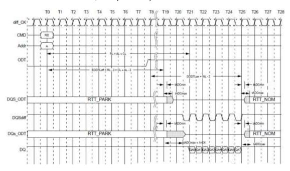
Example: CL=11, PL=0; AL=CL-1=10; RL=AL+PL+CL=21; CWL=9; DODTLon= AL+CWL-2=17; DODTLoff=AL+CWL-2=17;2tCK preamble)
