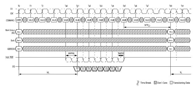
NOTE 1 tWTR\_L: delay from start of internal write transaction to internal READ command to the same bank group. When AL is non-zero, the external read command at TbO can be pulled in by AL.
