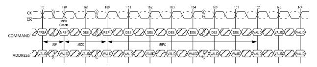
NOTE 1 Multipurpose registers Read/Write Enable (MR3 A2 = 1). Redirect all subsequent read and writes to MPR locations.
