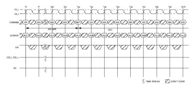
NOTE 1 Address setting: BA1 and BA0 indicate the MPR location A [7:0] = data for MPR A10 and other address pins are "Don't Care"
