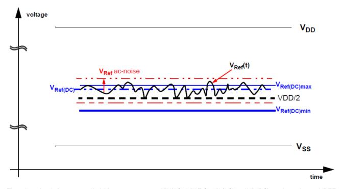
The voltage levels for setup and hold time measurements VIH(AC), VIH(DC), VIL(AC) and VIL(DC) are dependent on VREF. "VREF" shall be understood as VREF(DC), as defined in Illustration of V.
