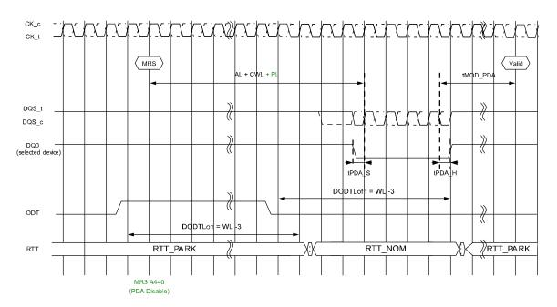
NOTE RTT\_PARK = Enable; RTT\_NOM = Enable, Write Preamble Set = 2tCK and DLL = ON, CA parity is used
