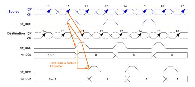
DQS - DQS driven by the controller during leveling mode must be terminated by the DRAM based on the ranks populated. Similarly, the DQ bus driven by the DRAM must also be terminated at the controller.
