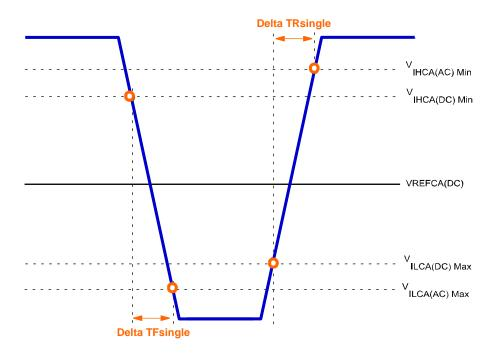
NOTE1 Single-ended input slew rate for rising edge = {VIHCA(AC)Min - VILCA(DC)Max} / Delta TR single
