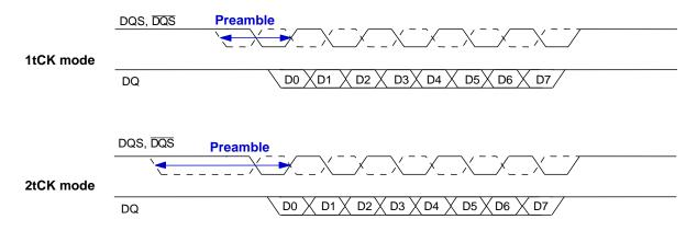
When operating in 2 tCK Write preamble mode in MR2 CWL (CAS Write Latency), CWL of 1st Set needs to be incremented by 2 nCK and CWL of 2nd Set does not need increment of it. tWTR must be increased by one clock cycle from the tWTR required in the applicable speed bin table. WR must be programmed to a value one or two clock cycle(s), depending on available settings, greater than the WR setting required per the applicable speed bin table.
