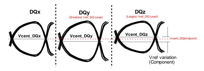
Vcent\_DQ(midpoint) is defined as the midpoint between the largest VREFDQ voltage level and the smallest VREFDQ voltage level across all DQ pins for a given DRAM. Each DQ pin's VREFDQ is defined by the center, i.e. widest opening, of the cumulative data input eye as depicted in below. This means a DRAM's level variation is accounted for within the DRAM Rx mask. The DRAM VREFDQ level will be set by the system to account for Ron and ODT settings.
