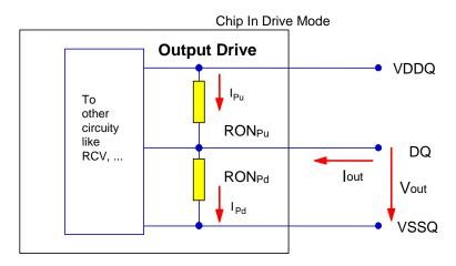
The individual pull-up and pull-down resistors (RONPu and RONPd) are defined as follows:
