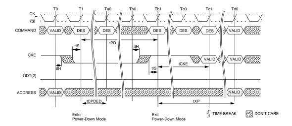
NOTE 1 Valid commands at T0 are ACT, DES, or PRE with one bank remaining open after completion of the PRECHARGE command.
