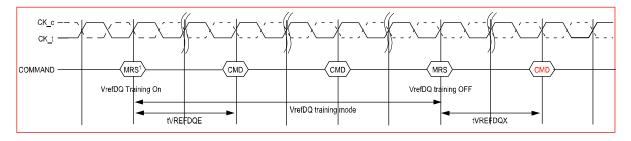
The MR command used to enter VrefDQ Calibration Mode treats MR6 A [5:0] as don't care while the next subsequent MR command sets NOTE 1 VrefDQ values in MR6 A[5:0]
