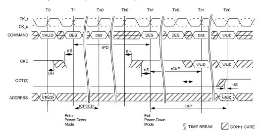
NOTE 1 Valid commands at T0 are ACT, DES, or PRE with one bank remaining open after completion of the PRECHARGE command.
