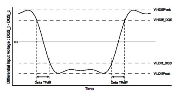
NOTE 1 Differential signal rising edge from VILDiff\_DQS to VIHDiff\_DQS must be monotonic slope.
