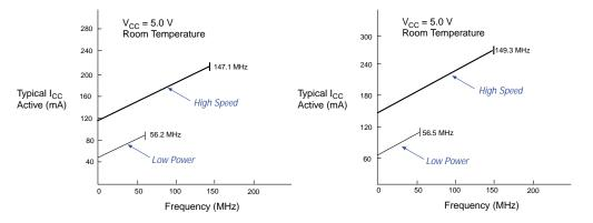
Figure 15.  $I_{CC}$  vs. Frequency for MAX 7000S Devices (Part 2 of 2)
