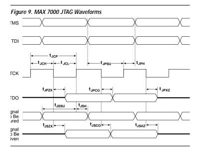
Figure 9 shows the timing requirements for the JTAG signals.
