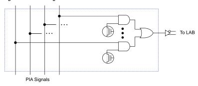
While the routing delays of channel-based routing schemes in masked or FPGAs are cumulative, variable, and path-dependent, the MAX 7000 PIA has a fixed delay. The PIA thus eliminates skew between signals and makes timing performance easy to predict.
