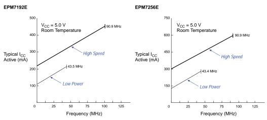
Figure 15 shows typical supply current versus frequency for MAX 7000S devices.
