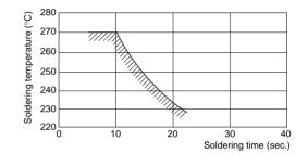
In case of repeated soldering, the accumulated Soldering time must be within the range shown above.
