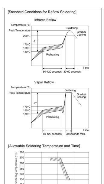
In case of repeated soldering, the accumulated Soldering time must be within the range shown above.
