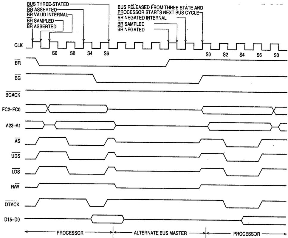
**Figure 5-24. 2-Wire Bus Arbitration Timing Diagram—Special Case**
