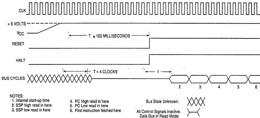
**Figure 5-30. Reset Operation Timing Diagram**
