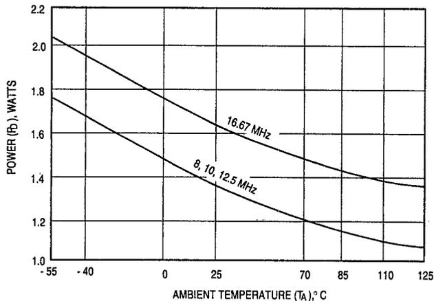
**Figure 10-1. MC68000 Power Dissipation (PD) vs Ambient Temperature (TA)
