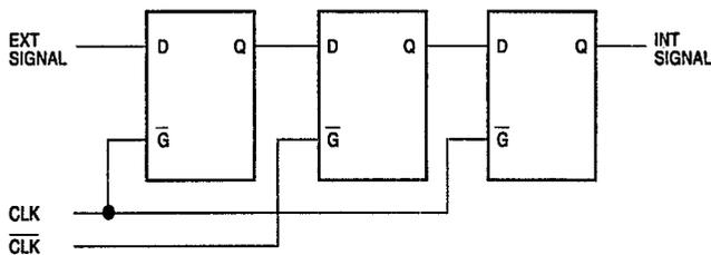
**Figure 5-37. Input Synchronizers**
