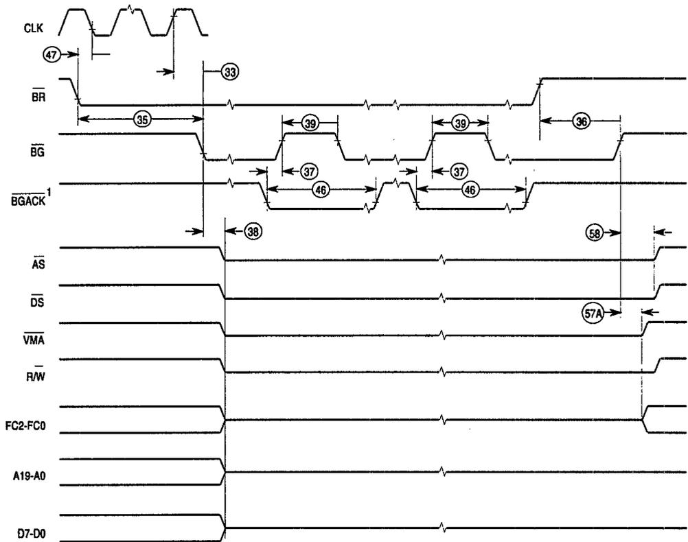
NOTES: Waveform measurements for all inputs and outputs are specified at: logic high 2.0 V, logic low = 0.8 V.
