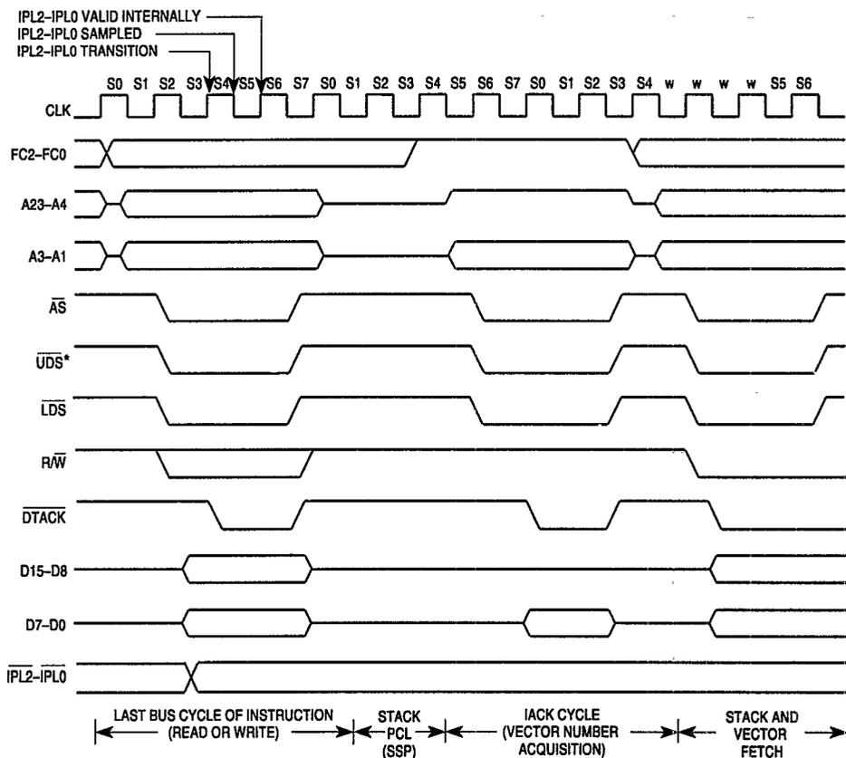
\* Although a vector number is one byte, both data strobes are asserted due to the microcode used for exception processing. The processor does not recognize anything on data lines D8 through D15 at this time.
