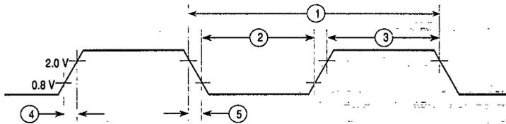
NOTE: Timing measurements are referenced to and from a low voltage of 0.8 V and a high voltage of 2.0 V, unless otherwise noted. The voltage swing through this range should start outside and pass through the range such that the rise or fall will be linear between 0.8 V and 2.0 V.
