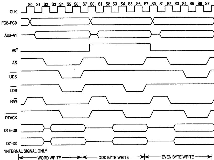
**Figure 5-7. Word and Byte Write-Cycle Timing Diagram**
