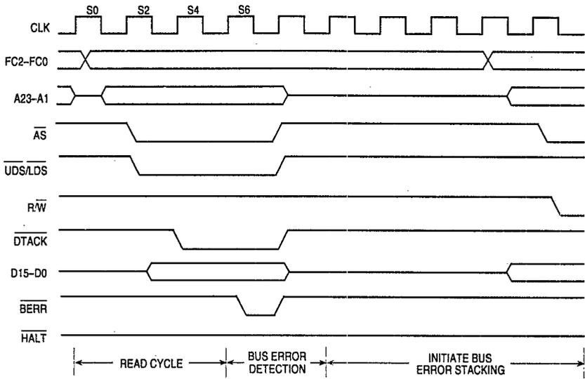
**Figure 5-26. Delayed Bus Error Timing Diagram (MC68010)**
