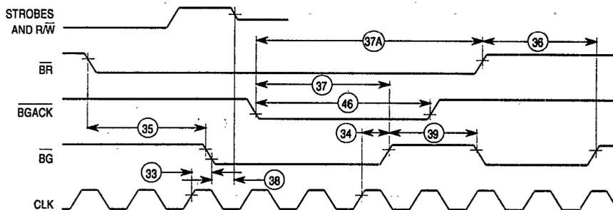
NOTE: Setup time to the clock (#47) for the asynchronous inputs  $\overline{\text{BERR}}$ ,  $\overline{\text{BGACK}}$ ,  $\overline{\text{BR}}$ ,  $\overline{\text{DTACK}}$ ,  $\overline{\text{IPL2-IPL0}}$ , and  $\overline{\text{VPA}}$  guarantees their recognition at the next falling edge of the clock.
