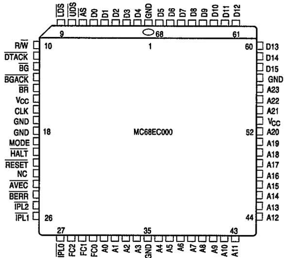
Figure 11-3. 68-Lead Quad Pack (1 of 2)
