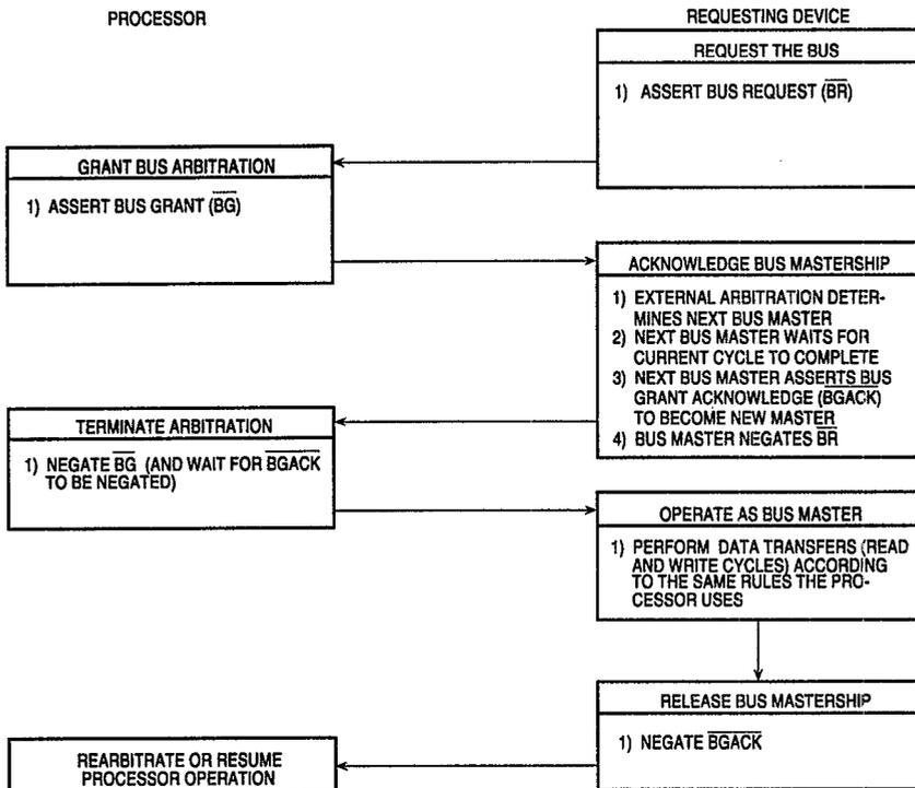
**Figure 5-13. 3-Wire Bus Arbitration Cycle Flowchart
