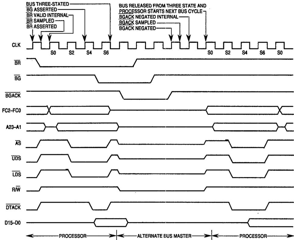
**Figure 5-21. 3-Wire Bus Arbitration Timing Diagram—Special Case**
