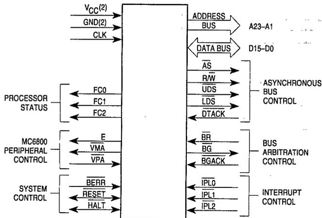
**Figure 3-1. Input and Output Signals
