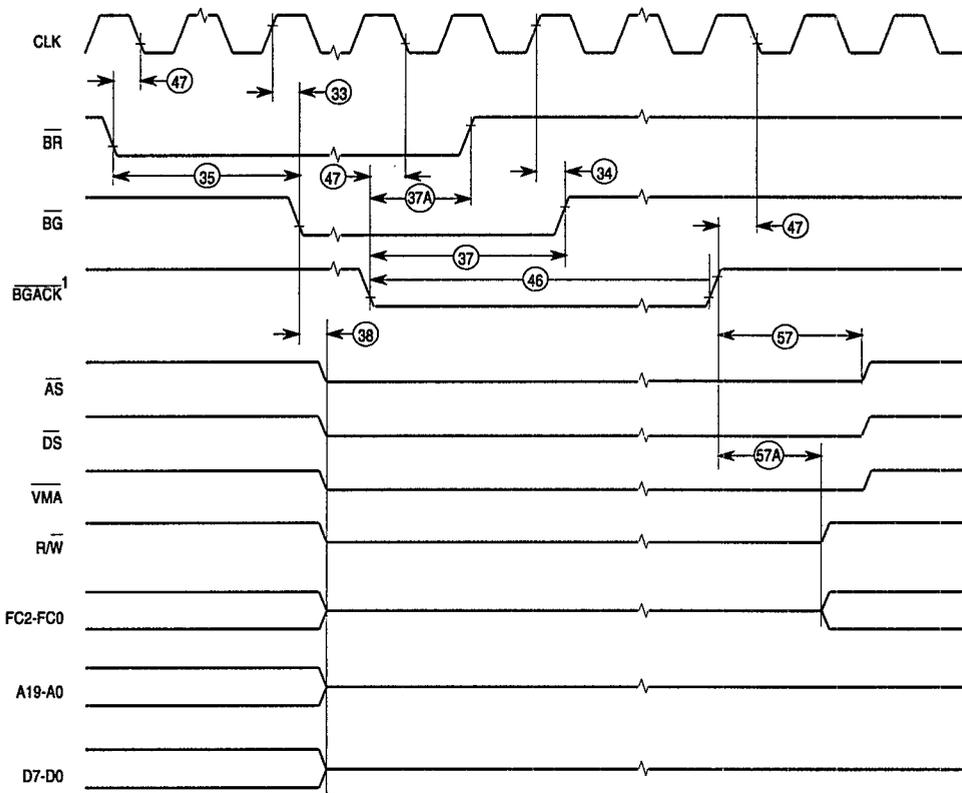
NOTES: Waveform measurements for all inputs and outputs are specified at: logic high 2.0 V, logic low = 0.8 V.
