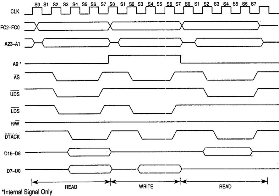
**Figure 5-4. Word and Byte Read-Cycle Timing Diagram**
