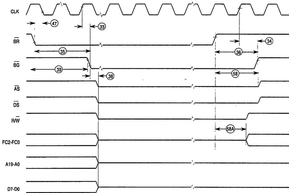
NOTES: Waveform measurements for all inputs and outputs are specified at: logic high 2.0 V, logic low = 0.8 V.
