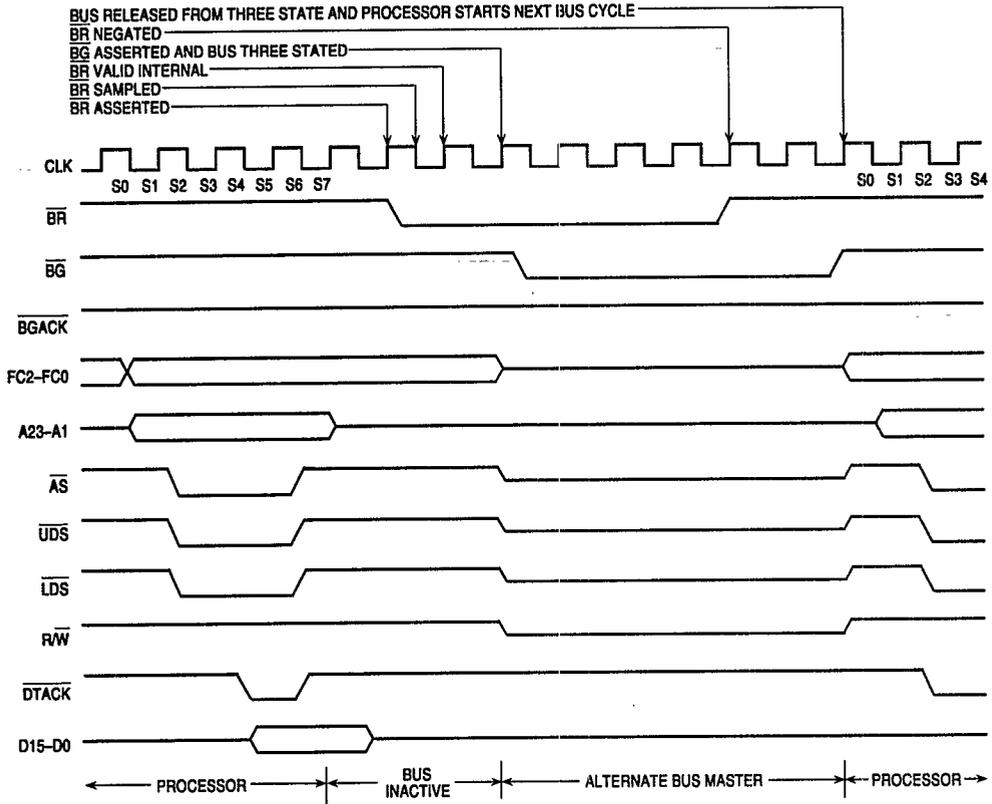
**Figure 5-23. 2-Wire Bus Arbitration Timing Diagram—Bus Inactive**
