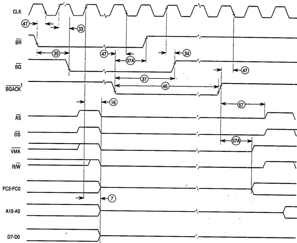
NOTE: Waveform measurements for all inputs and outputs are specified at: logic high 2.0 V, logic low = 0.8 V.
