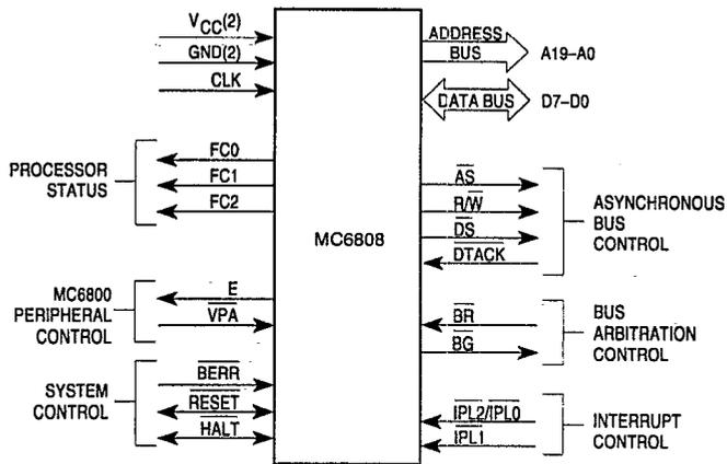
Figure 3-4. Input and Output Signals (MC68008, 48-Pin Version)
