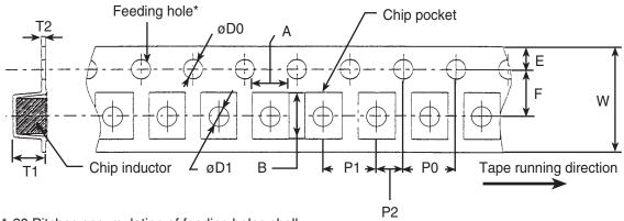
$^{\star}$  20 Pitches accumulation of feeding holes shall be 80  $\pm$  0.15 mm.
