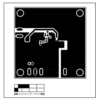
Figure 4. MAX1873 EV Kit PC Board Layout—Solder Side
