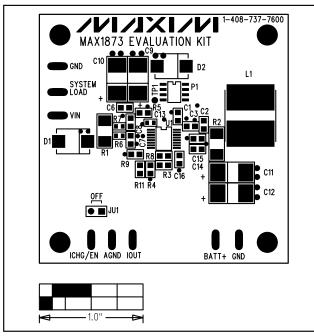
Figure 2. MAX1873 EV Kit Component Placement Guide— Component Side
