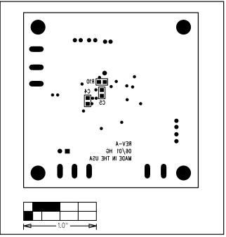
Figure 5. MAX1873 EV Kit Component Placement Guide—Solder Side
