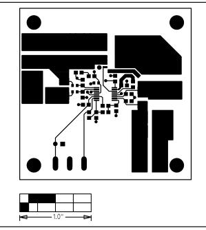
Figure 3. MAX1873 EV Kit PC Board Layout—Component Side
