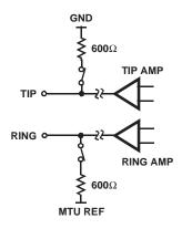
FIGURE 3. LPS 2-WIRE INTERFACE CIRCUIT DIAGRAM
