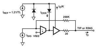
FIGURE 2. CURRENT LIMIT FUNCTIONAL DIAGRAM
