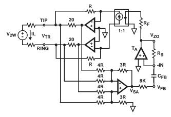
FIGURE 11. IMPEDANCE SYNTHESIS
