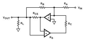
FIGURE 4. VOLTAGE FEED CURRENT SENSE DIAGRAM
