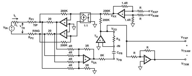
FIGURE 13. SCHEMATIC FOR 2-WIRE TO 4-WIRE GAIN DERIVATION
