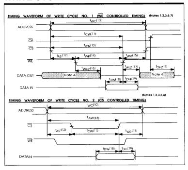
Writing to the S128K8 is achieved when the chip select (CS) and write enable (WE) inputs are LOW. Data on the input/output pins is written into the memory location specified on the address pins (A0-A16).
