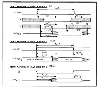
Reading the S128K8 device is accomplished by taking chip select (CS) and output enable (OE) LOW, while write enable (WE) remains inactive or high. Under these conditions, the contents of the memory location specified on the address pins will appear on the appropriate data input/output pins.
