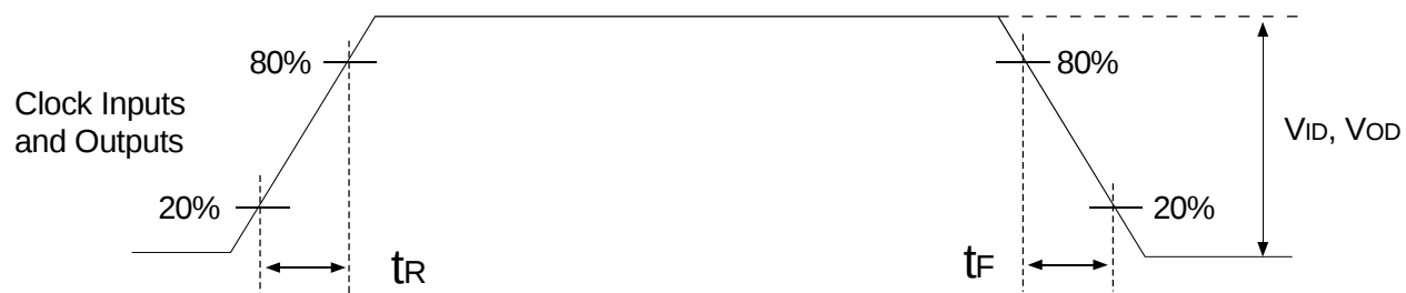
Figure 8. Input and Output Slew Rates
