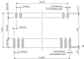
Recommended metal mask thickness: t = 0.1 mm
