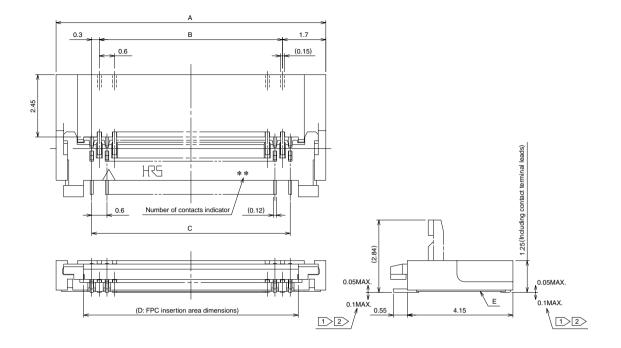
Notes 1 The coplanarity of each terminal lead is within 0.1.
