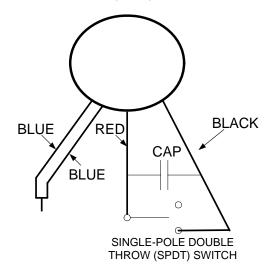
Capacitors are non-polarized and must always be connected between the red and black leads. Always connect the (2) coil blue leads together. Connect the power supply to the blue leads and red lead to produce clockwise (CW) rotation viewing shaft end. Connect the power supply to the blue leads and black lead to produce counter-clockwise (CCW) rotation viewing shaft end.
