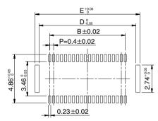
Recommended solder paste thickness: 120  $\mu$ m
