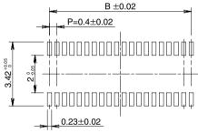
Recommended solder paste thickness: 120  $\mu \mathrm{m}$
