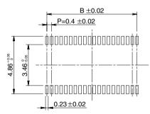
Recommended solder paste thickness: 120  $\mu \mathrm{m}$
